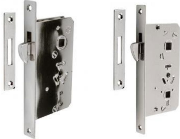
#18.3797 Entry Lock Skeleton Key Privacy Lock #18.9750 Sliding Door Lock; 37 mm (1 1/2) backset. Face plate: 160 x 15 x 2 mm; Lock case: 118 high x 65 wide x 12 mm thick. Center to Center PC: 59 mm Marine grade; stainless steel and brass chrome plated parts.
